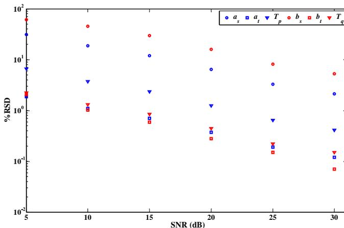
**Fig. 10.** Relative standard deviation of the load model estimates against SNR.
