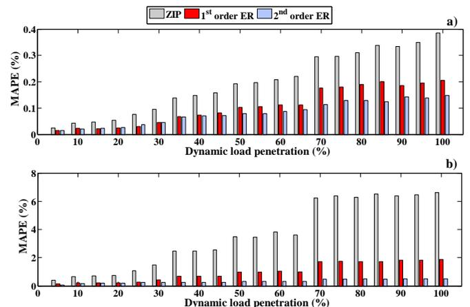
Fig. 5. MAPE for (a) real and (b) reactive power simulation using the three examined models.
