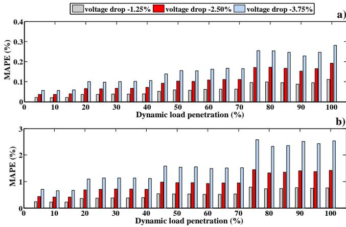
Fig. 6. MAPE of (a) real and (b) reactive power response for different disturbance levels – Simulations using the 1st order ER model.
