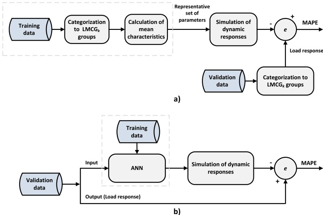
Fig. 9. Block diagram of cross-validation processes for the (a) mean characteristics and (b) ANN approaches.
