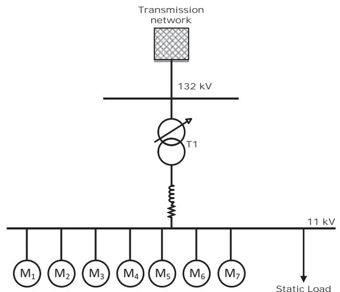
Fig. 4. One-line diagram of the substation modelled.
