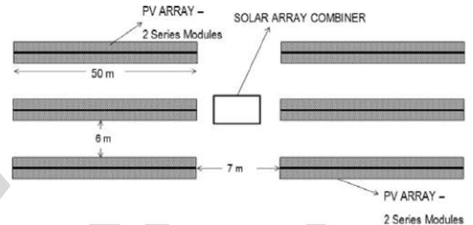
Fig. 6. Topology of the 150-kWp PV system.
