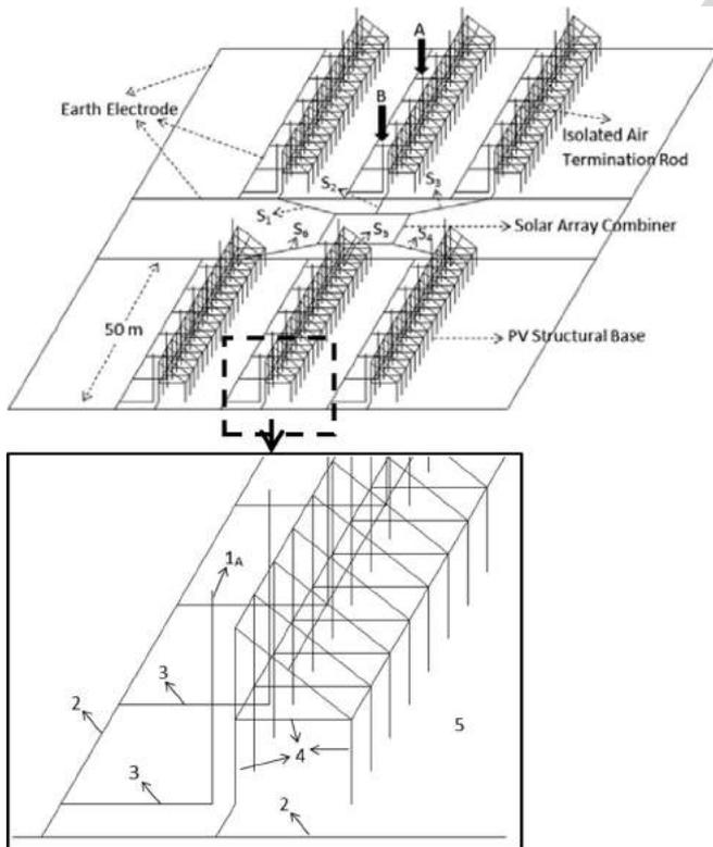
Fig. 11. Real-scale simulation model for a 150-kW solar park—with isolated L.P.S.
