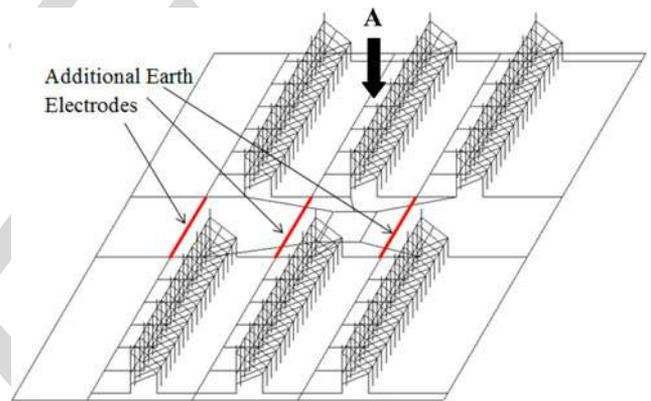
Fig. 17. Real-scale simulation model for a 150-kW solar park—with nonisolated L.P.S and additional earth electrodes to enhance the earthing system.
