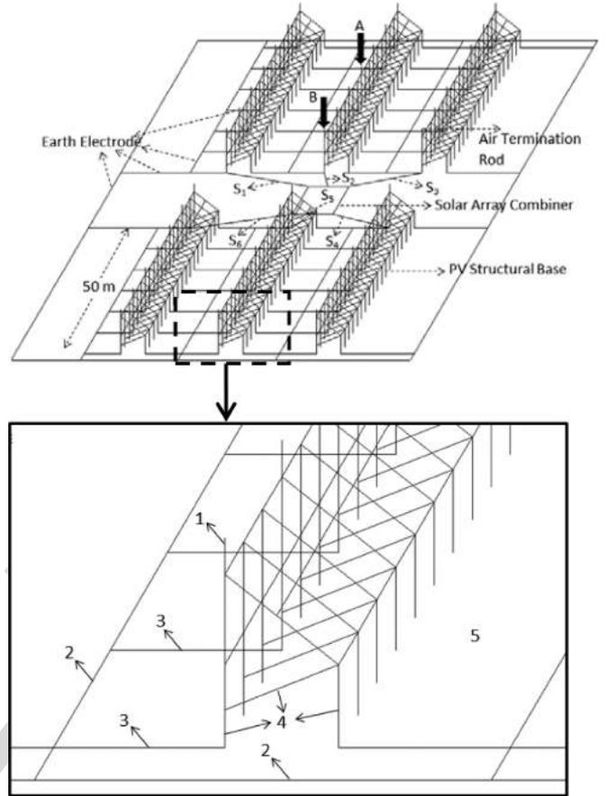
Fig. 9. Real-scale simulation model for a 150-kW solar park—with nonisolated L.P.S.
