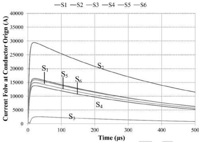
Fig. 13. Current flow ( $i_{s\_N}$ ) through the six dc strings—isolated L.P.S.
