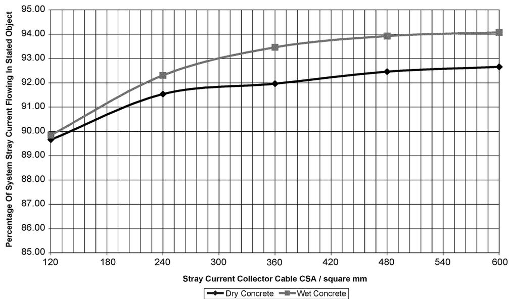
Fig. 12. Efficiency of the stray current collection system for wet and dry concrete.
