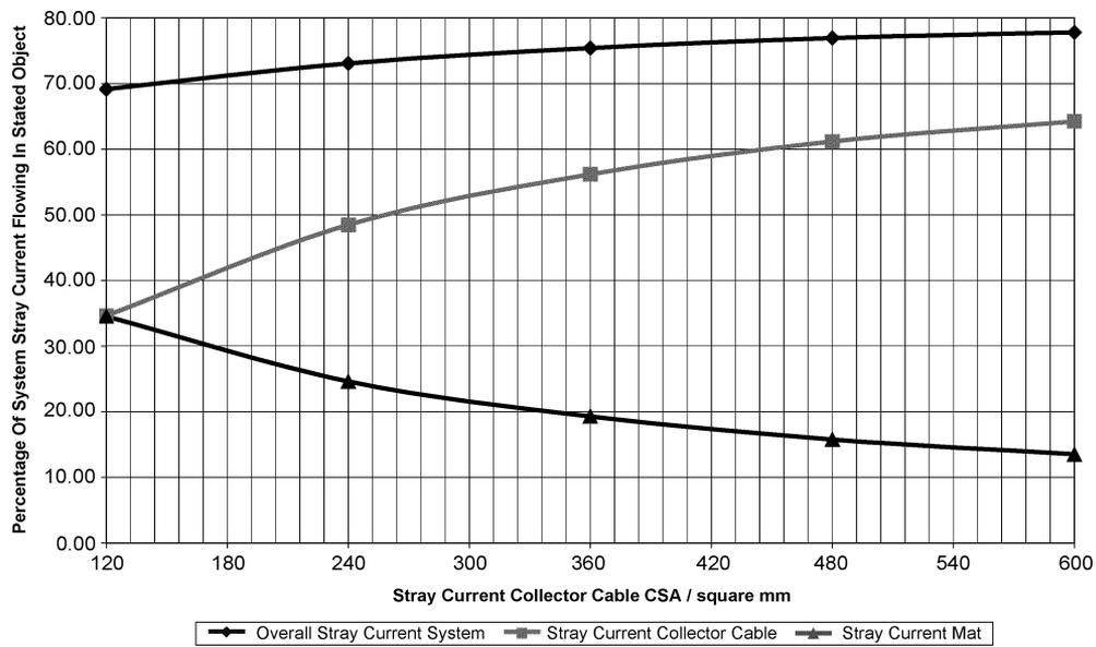
Fig. 11. Efficiency of the stray current collection system against stray current collector cable cross-sectional area (10 Ωm soil around the dry concrete base).
