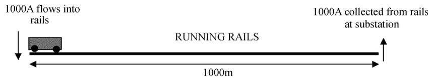
Fig. 1. Section of model to illustrate stray current production.
