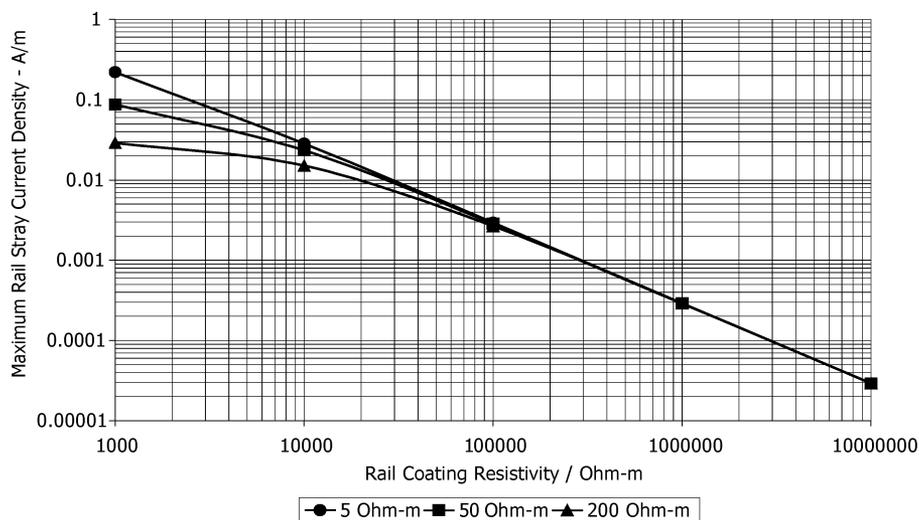
Fig. 6. Variation of maximum rail stray current density as a function of rail coating and base material resistivity.
