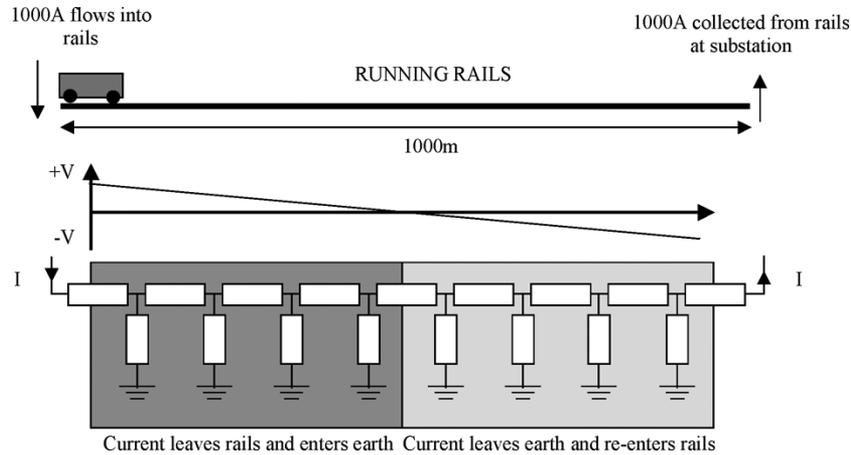
Fig. 3. Basic model of floating rail system, illustrating stray current leakage.
