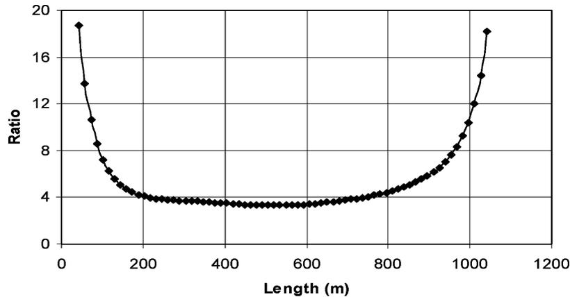
Fig. 5. Ratio of grounded to floating system summated positive stray current charge along the rail length.
