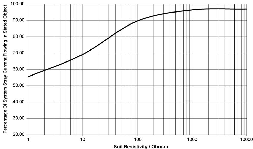
Fig. 10. Efficiency of the stray current collection system against soil resistivity.
