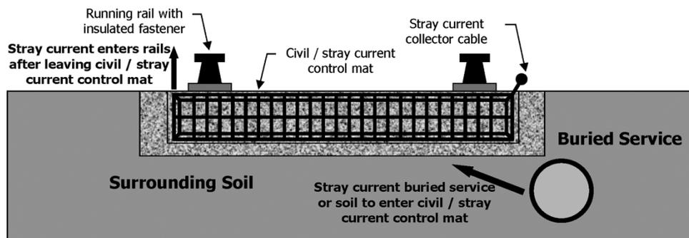
Fig. 8. Path of stray current returning to the running rails.
