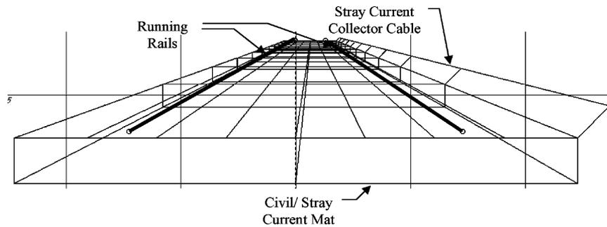
Fig. 9. CDEGS model of stray current collection system.
