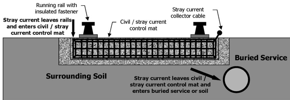
Fig. 7. Path of stray current leaving the running rails.
