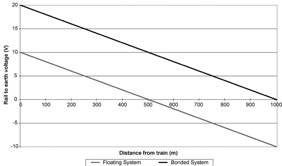
Fig. 2. Rail-to-earth voltage profiles for a floating and grounded rail system.
