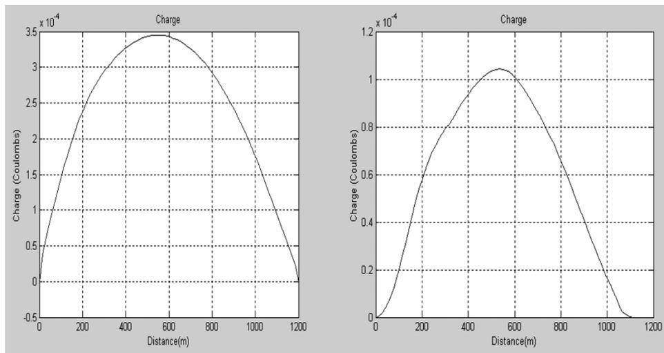
Fig. 4. Positive (corrosive) stray current charge from running rails in dynamic simulation of the (left) grounded and (right) floating system.
