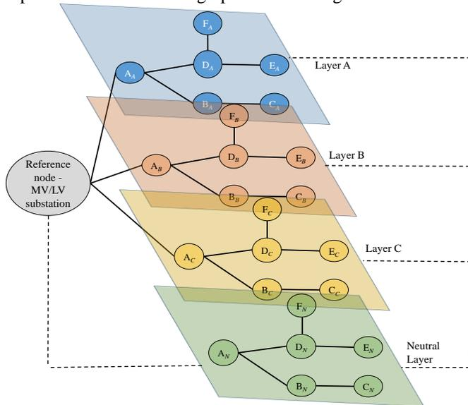
Fig. 2: Illustration of the (virtual) separation of three-phase, four-wire distribution networks into multiple layers.
