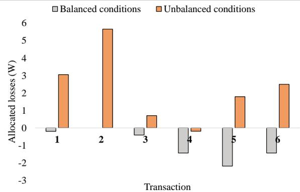
Fig. 5: Allocated losses to peer-to-peer transactions of Table XI for balanced and unbalanced conditions.
